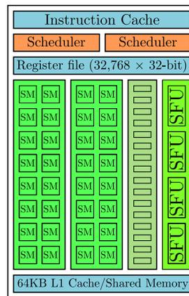
Figure 3. A single Streaming Multiprocessor [17]. 32 Streaming processors share a register file and shared memory. Four special function units (not considered here) compute transcendental functions at a reduced accuracy.
